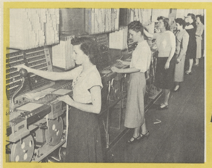
At terminal, the telegram is transmitted automatically to the office of delivery by the push of a button.
